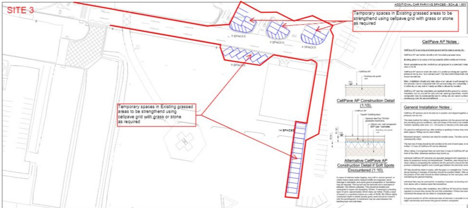
Temporary spaces in Existing grassed areas to be strengthened using cellpave grid with grass or stone as required
